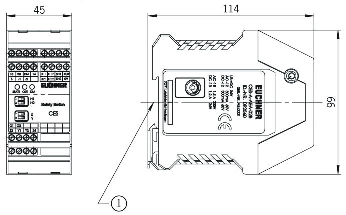
1 Suitable for 35 mm mounting rail according to EN 60715
