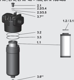
3.2 SPARE PARTS LIST LFN, LFNF 40 – 100 (2.0 VERSION); DFN, DFNF 40 – 100 (1.1 VERSION), DFN 160 - 400
